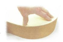
Carefully check fit of top on sides so that when just lightly pressed with fingers near the edge it will lay flat with no gaps. Sand more to correct fit if needed.
