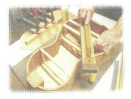
$6.\Box$  Gluing the back in place; use the same techniques as in gluing top on.
