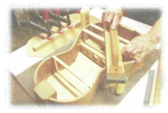
View of top with kerfing and braces in place and sanding done. Your kit will not call for as much kerfing or arc as this 3/4" arc Moriah model. Check plans for details.
