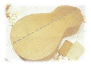
The top gets done in much the same way except for the area where key chest and tuning head attach on the angled end block. **Do not round over** edge on the area where key chest attaches at the head block and where tail piece attaches on the tail block area. This last picture shows the back with the decorative strip which is offered as an upgrade for an additional charge.
