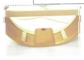
2.? Mark and drill for strap button screws in the vertical center of the sides and in center of width of the ply. Be careful to have the 3/32" drill enter the wood at a 90 degree angle and drill all the way through on both sides.
