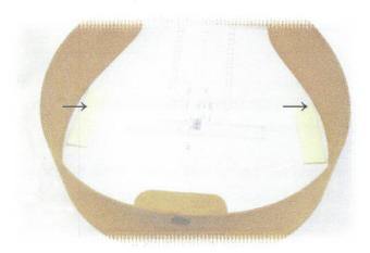
12. ☐ Starting with the bridge brace try your clamping method without glue first. If the fit is good, remove the brace, glue it with yellow glue and clamp it in place.
