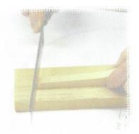
2. ? Cut brace sides & ¼" dowels for center of braces to correct length. Dowels should touch bottom of holes when properly sized and fitted together with brace sides. Each brace unit should measure about 4" tall when assembled. Unit should be dry fit before gluing with all joints tight fitting.
