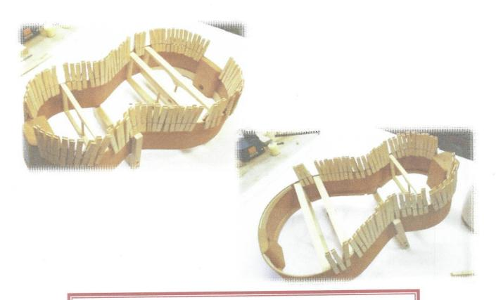
We recommend as pictured below, kerfing the bottom first; then turn the body over, move side retaining fixture, and glue kerfing to top edge between braces keeping it flush with edge.
