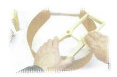
11.□ Put plastic wrap over plans to protect from glue. Set body
