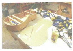
All parts that touch the back get glued – braces, sides, kerfing, & end blocks.
