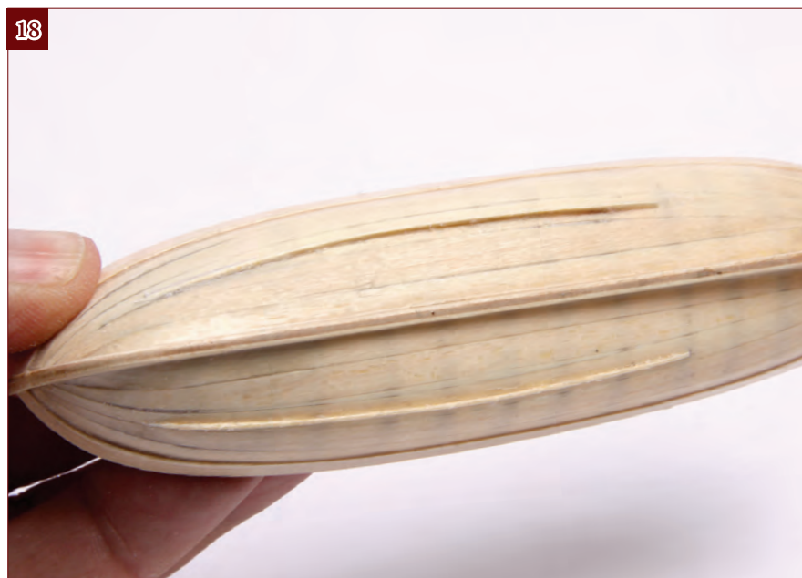
18. The finished result should look like this. If you opted for a painted finish, the hull will be patched with filler/primer, but you will apply a smooth white paint at the next stage.
