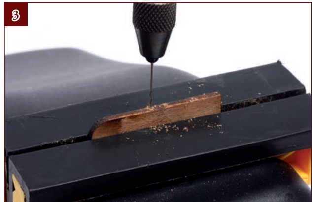
3. Clamp the wooden base in a modelling vice and use a micro drill to drill the four holes in the side of the base. The wire-gauge drill bit needs to be a fraction larger than the shaft of an eyebolt.
