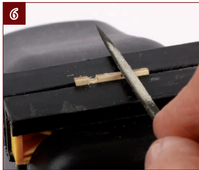
6. Use a needle to file the notches to a depth of 1.5-2 mm.
