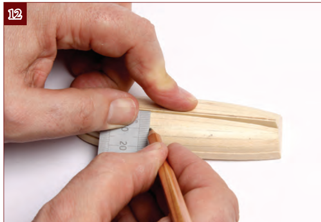
12. They run forward to 13 mm from the bows, curving out in the middle so they are 11 mm away from the keel at the centre point.
