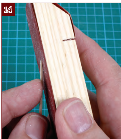
14. Lightly sand both ends of two of the strips so that they taper from one side and are widest in the middle.
