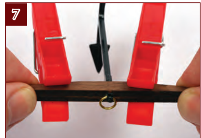
7. Press the two halves together around the shank, ensuring that they line up with each other. Clamp lightly (clothespins are a simple alternative to clamps or a vice) and leave to dry thoroughly.
