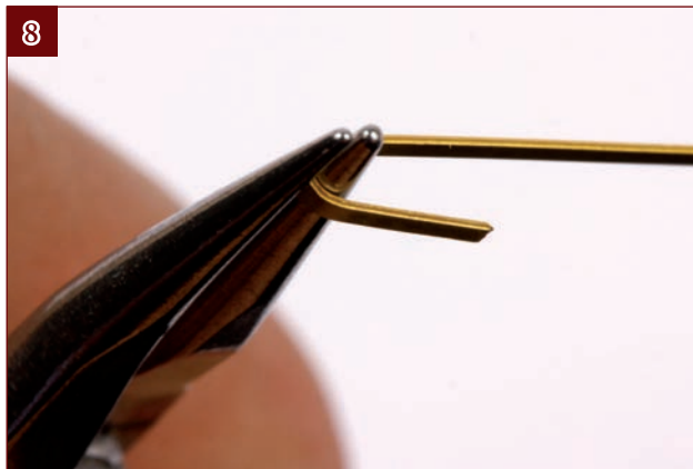
8. Take the brass strip and use needle-nose pliers to form a 2-mm bend about 5 mm from one end.
