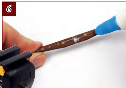
6. Apply glue sparingly to one half of the stock. Apply a little to both the central slots.
