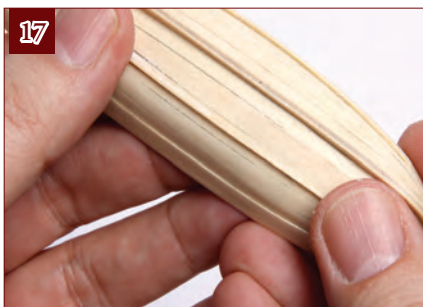
17. Press the rubbing strips into place, following the lines you marked in Steps 11-12, and hold until the glue sets.
