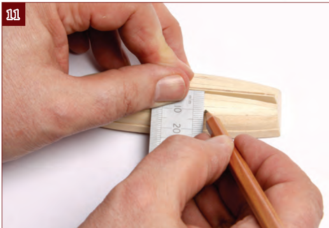
11. Mark the position of the rubbing strips. They start 25 mm forward of the transom, 9 mm away from the keel.
