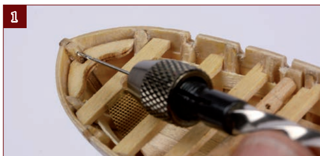
1. Drill a hole inside the end of the keel just above the bow brace, using a bit the same size as the eyebolt (0.5mm/No. 74).
