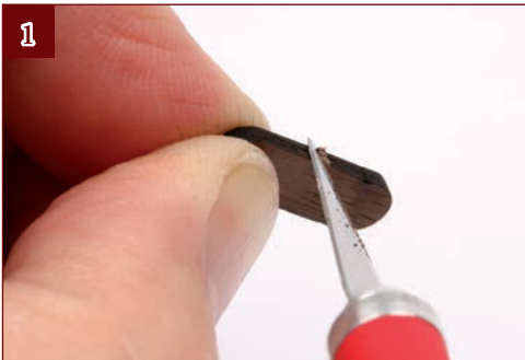
1. Use a craft knife to shave off any whiskers of wood attached to the three larger wooden components.
