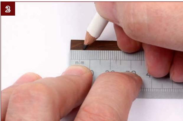
2. Following the diagrams at the top of page 14, mark the positions of the holes in the side of the wooden base and mark where the base, the rounded slide that goes on top, and the square mounting platform that goes under it fit together.
