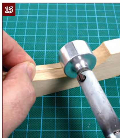
15. Gently bend the strips along their thin edge so that they fit the curve of the hull, as shown in Steps 16-17.
