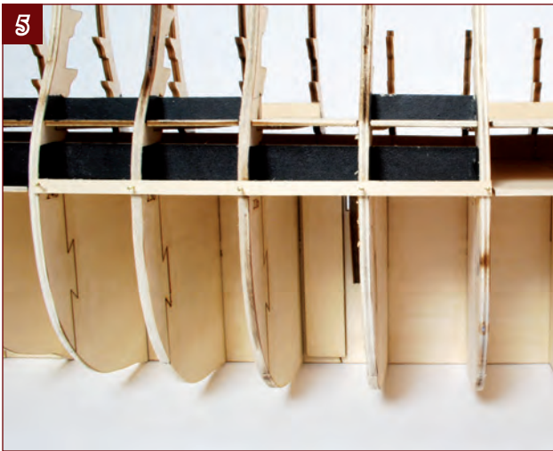
5. Start the fifth layer of planks with a plank fitted between frames 16 and 23.
