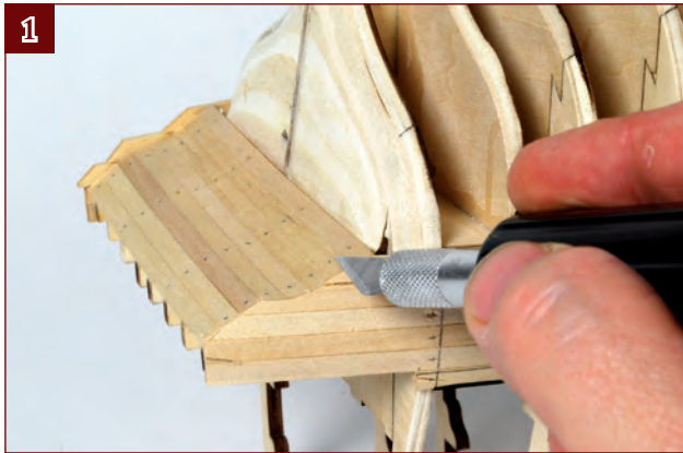
1. Carefully trim the overhanging ends of the planks with a sharp knife. They should finish flush with the gallery supports.
