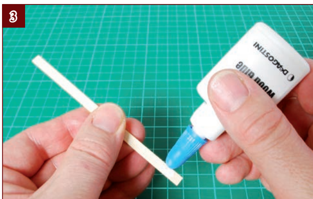
3. Apply glue where the plank contacts the bow formers 7.
