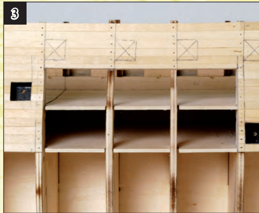
1. Mark the vertical lines along the side of each frame in the cutaway area as shown.
