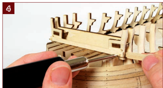
4. Now pin the plank in place, holding the support directly behind the nail. Do not push the pin home, as this will also nail the support in place.
