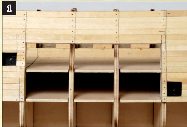
1. Mark the vertical lines along the side of each frame in the cutaway area as shown.
