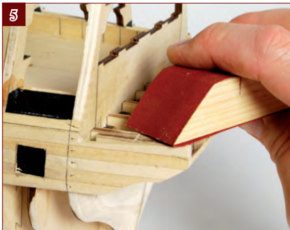
5. Finally, use sandpaper to bring the plank flush with the top of the gallery support. When you have finished, the planks should be flush with the gallery support at the top, bottom and end, as shown on the right.
