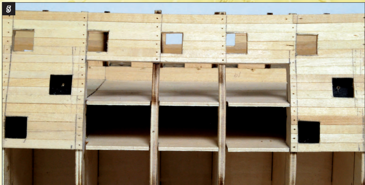
5. After you have finished cutting the gun ports above the cutaway section, your hull should look like this.
