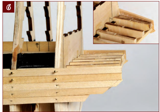
6. Complete this layer of planks. Note that the fifth plank overhangs the end of the gallery supports, and that the top of the plank sits above the level of the supports. It will be sanded down later, but leave it for now.
