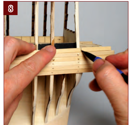
8. Cut the rear plank so that it overhangs the last frame by 1 or 2 mm.
