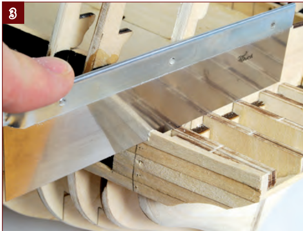
3. Carefully cut the planks flush with frame 30, using a razor saw. Be sure to stop when the saw gets to the tops of the gallery supports.
