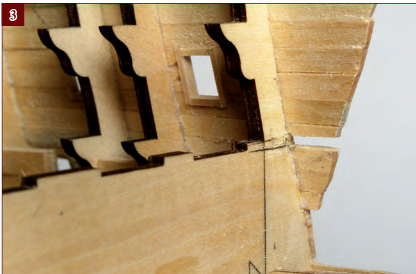
1. Glue the two supports (59) to the upper false deck (58), making sure they are the right way round, square and upright.
