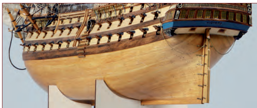
The complex curves of the stern planks require some tight bends where they sweep up over the transom.
