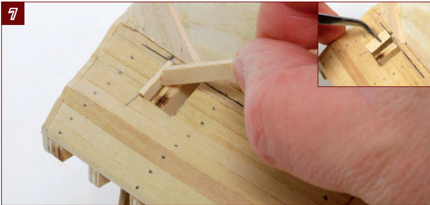
7. The stern gun ports are completed in a similar fashion. You should be able to use your jig to cut the planks to approximate length. First trim the side pieces to fit, and glue one of them in position.
