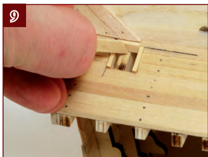
9. Trim the lining nearest the transom to size, and glue it in place. It will butt up to the exposed gallery support.
