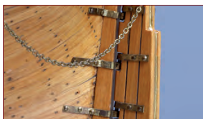
The complex curves of the stern planks require some tight bends where they sweep up over the transom.
