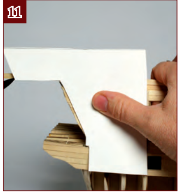
11. Fit another plank from frame 25 to the stern of the model. Depending on the tapering of the planks below, this will probably need to go to the extended section of the template. If even part of the plank reaches this length, do not cut it to the shorter part of the template.
