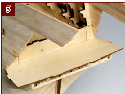
5. Now test-fit the lower false deck in place. Do not force it if it is a tight fit.
