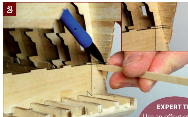
2. You need to cut slots in the stern planking for the upper false deck. Extend lines from the top of the transom and the notches in it as shown.
