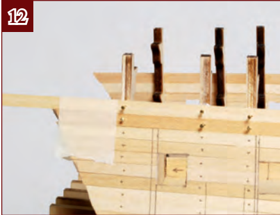
12. Fit this plank using glue and pins as usual. The aft section of the plank can be held with masking tape or a clothespin (see Step 4).
