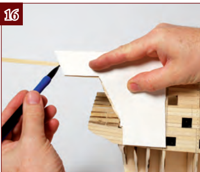
16. Again, use the template to ensure that the plank is the correct length before cutting.
