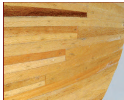
Examples of "dropper planks" at the bow, where two tapering planks stop short and are finished with a short, single plank.
