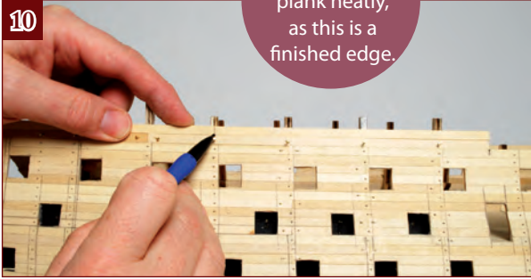
10. Fit the next plank from the pencil mark to the centre of frame 25.
