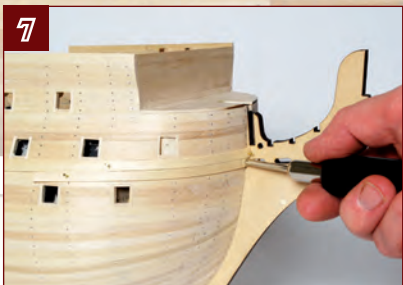
7. Add another 1 x 5-mm strip under the first, running from the bow to stop at frame 14.
