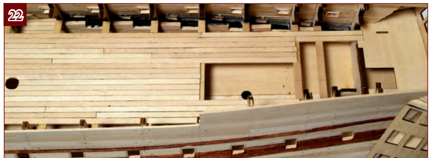
22. Lay two rows of planks from the bow all the way back onto frame 30 and the upper false deck of the rear gallery. Repeat this on the both sides of the deck.
