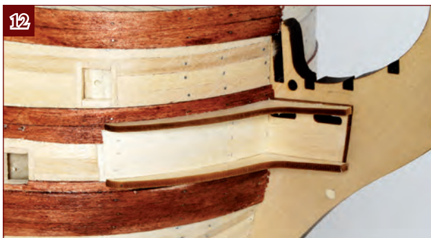
12. Fit a second dolphin as in Steps 5 and 6, then glue it in position. It should butt up against the planks laid in Step 9.
