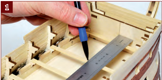
1. Using a rule, mark the centre line on the deck support beams. Use the line previously drawn on frame 12, the forward bulkhead, as a guide.
