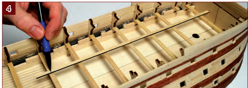
4. Lay a plank along the lines you marked in Step 2, with one end against frame 12. Draw a line across in line with the centre of frame 20.
