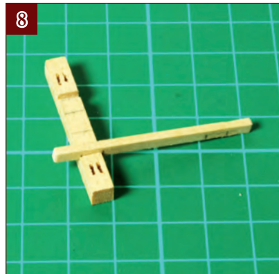
8. Test-fit the crossbeam in each slot. It should be a snug fit. If it's too tight, ease the slots slightly using a needle file.
