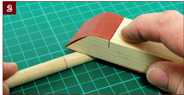
2. Sand two flats from the end up to the line, until the dowel is a smooth sliding fit in the angled slot for the bowsprit in the false keel.
