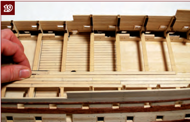
19. With the 303-mm gauge held against frame 12, lay a plank from the end of the gauge to the centre of frame 25.
