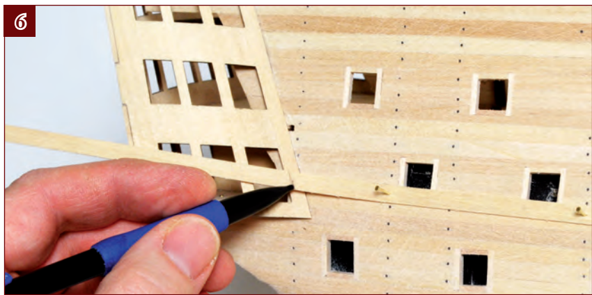
6. Mark the end of the strip, allowing a few millimetres excess, and cut it to length. Keep the offcut for planking the bow deck.
