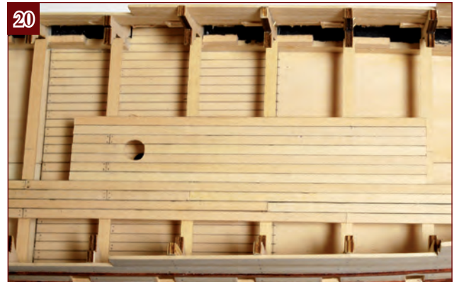
20. Repeat this with a further six planks, making a hole for the main mast in the same way as you did for the foremast.
