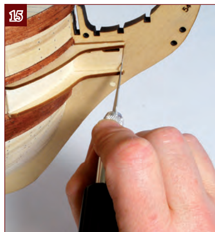
15. Trim the front of the dolphins, so the ends are flush with the front of the stem reinforcement.
