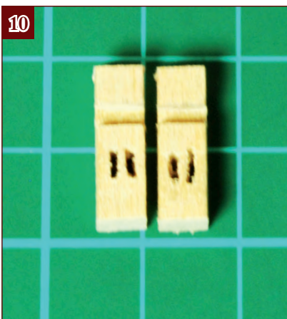
7. Use a craft knife to remove the wood between each pair of saw cuts, forming the two slots.
