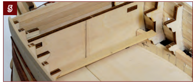
5. Glue the strip across the lowest support brackets on frame 13, with the brackets positioned in the centre of the width. If the strip is a tight fit, don't force it, as any bowing will make it hard to fit the deck planking. Trim a little off, and try again.
