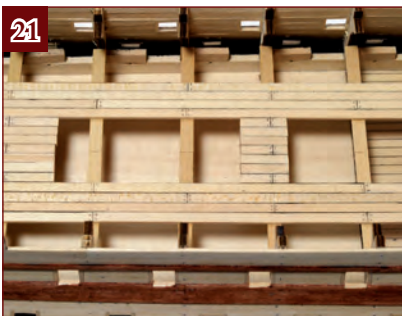
21. Lay four rows of planks from the bow to frame 27 on the starboard side in the same way as you did on the port.
