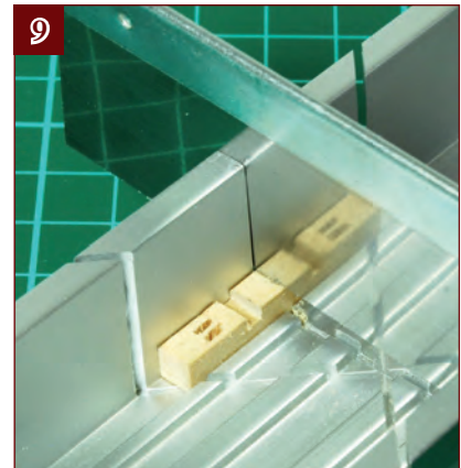
9. Saw the uprights to their finished length of 17 mm.
