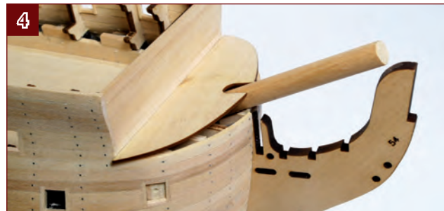
4. Try the bow deck in position. It will not lay flush until the "U"-shaped slot is enlarged.
