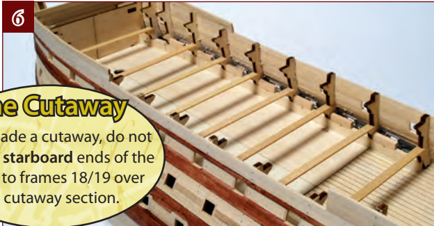
6. Repeat the process to fit deck support beams across all the frames except frames 14 and 26.
