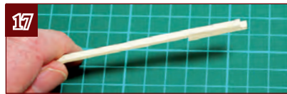
17. Glue a small strip of wood to extend the end of a 300 mm plank to make a gauge 303 mm long.
