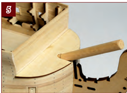
5. Gradually enlarge the slot (keeping the rounded end), until the deck sits flush on the tops of the bow formers.
