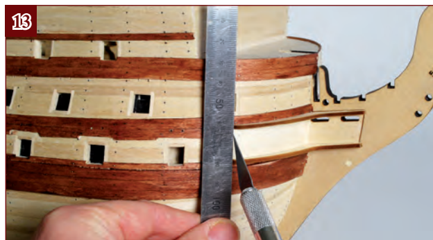
13. Take a straightedge and a sharp knife, and mark a line along the planks between the ends of the two dolphins.
