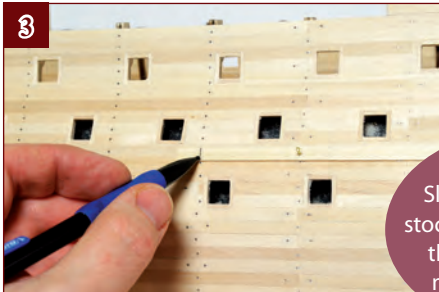
3. Mark the end of the strip so it lands on a frame, and cut it to length.
