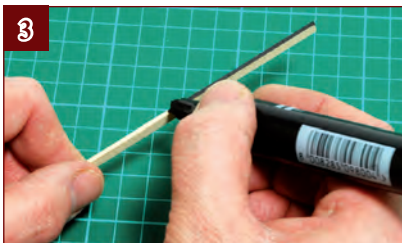
3. You can simulate the caulking lines by running a black marker pen down one side of the deck planks, in the same way as you did on the bow decks.
