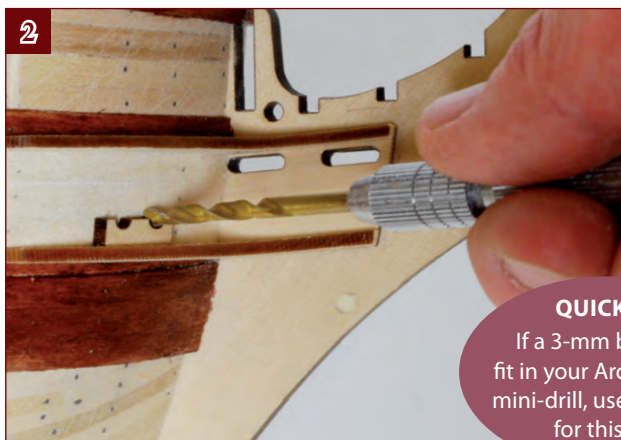
2. Drill the two hawseholes above the semicircular cutouts in the reinforcement, using a 3-mm drill bit.
