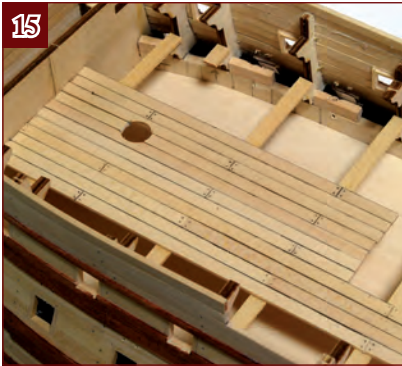
15. Add another three planks, each 140 mm long, cutting an arc in the first one to complete the hole for the mast.
