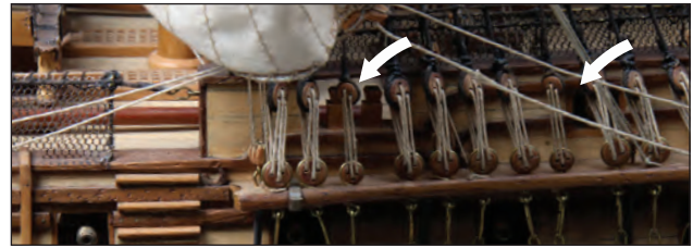
The two posts of the timber heads, and the first gun port (arrowed), behind the rigging on the finished model.
