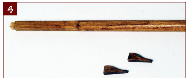
4. If you have chosen a natural wood finish, stain the main mast and bibbs dark oak (or a colour of your choice).
