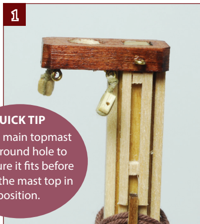
1. Glue the mast cap in position. Make sure it is straight and square. Also make sure that the round hole is directly above the square hole in the main top.
