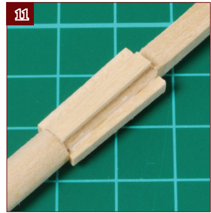
11. Cut four pieces of 2 x 3-mm wood to fit the octagon. Chamfer the edges, glue them in place and allow to dry.
