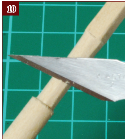
10. Carve an octagonal base for the cross tree support.
