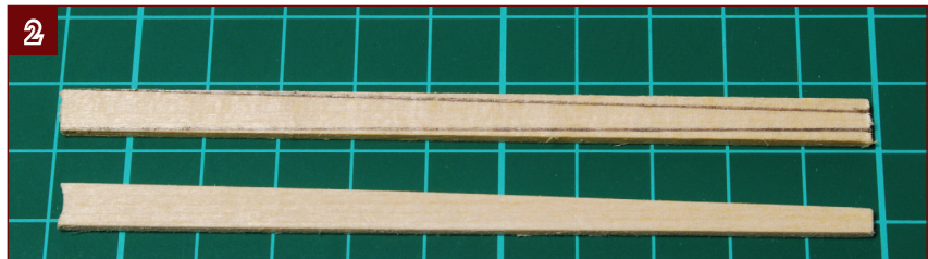
2. Cut two pieces of 2 x 6-mm wood, each 106 mm long. Draw pencil lines starting the full width of the plank at one end and ending 3 mm apart at the other. Sand both pieces to a smooth taper from 6 mm to 3 mm. Then sand an arc in the wider end to match the radius of the hounds made in the previous step.
