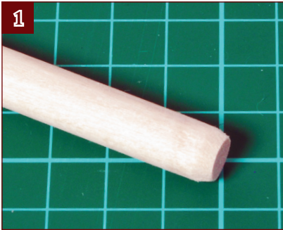
1. Sand a small bevel on the bottom of the mast.
