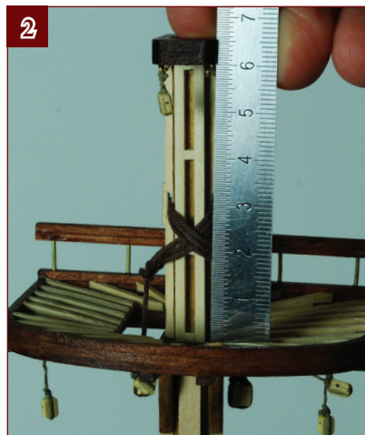
2. Measure the distance from the main top cross tree (which is glued to the mast) to the underside of the mast cap.
