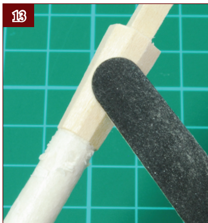
13. Use an emery board (nail file) to taper the mast support. Use the plan as a guide to get the correct shape.
