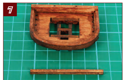
7. Glue one 2 x 3-mm strip to the rear of the top, and glue the other to the 2 x 2-mm strip to form the handrail. If you are staining the model, stain the assembly to match the other tops.
