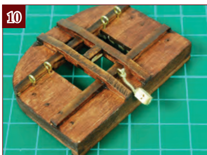
10. Use a short length of thread to add a 5-mm double block to the rear eye.
