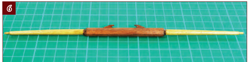
6. Stain the yard to match the other yards already constructed. If you are painting the yard, leave it until after the next step.
