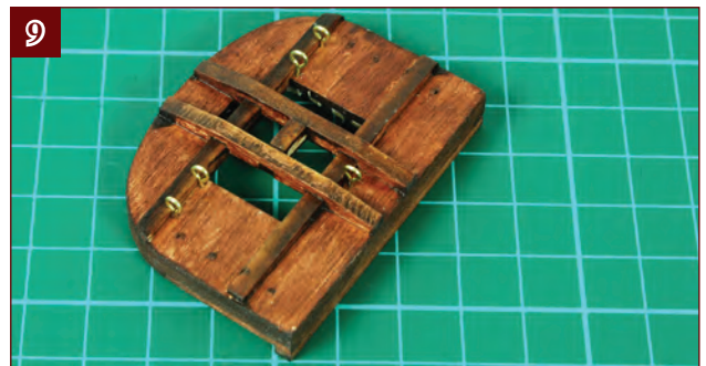
9. Turn the top over and glue five brass eyebolts as shown, after shortening their shanks to 3-4 mm.
