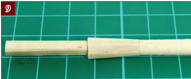
9. Use the 2 x 3-mm wood to complete the cross tree supports. The technique is described fully in Stage 63.
