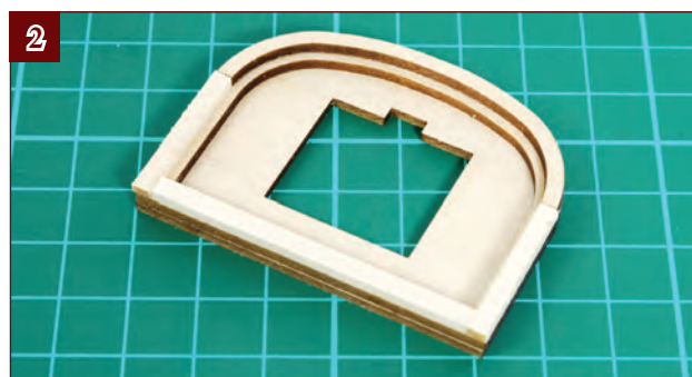
2. Complete the top border using 2 x 3-mm strip. Make sure the inside edge of the strip lines up with the inside edge of the curved, laser-cut border. It does not matter if the outside edge overhangs slightly.
