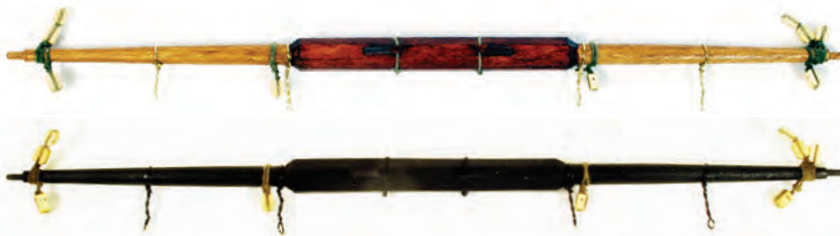
7. Add the two rope bindings using the 0.25-mm thread, and add the four footrope supports. The technique for fitting these is described in Stage 65. If you are painting the yard it should be painted black now.
