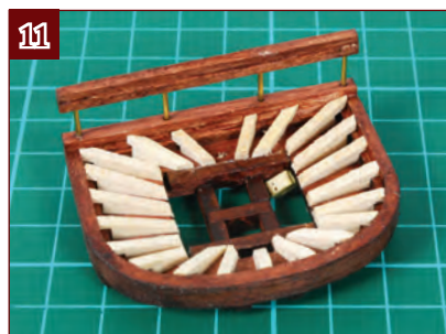
11. Cut four lengths of brass wire, about 12 mm long, to fix the handrail.
