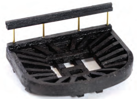
9. Turn the top over and glue five brass eyebolts as shown, after shortening their shanks to 3-4 mm.
