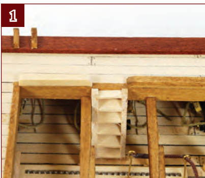
1. Cut two lengths of 3 x 3-mm wood to fit the side of the opening, running between the ladder and the end rail. Sand a radius on the ends by the ladder.
