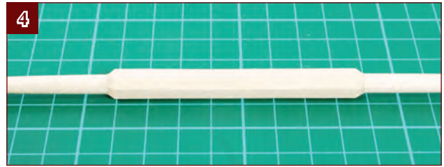
4. Complete the centre section bracing using strips of 4 x 2-mm wood. The technique is fully described in Stage 65.
