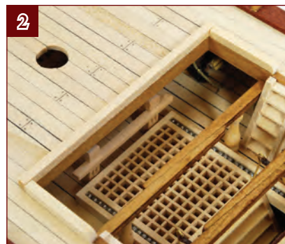
2. Cut a length of 3 x 3-mm wood to fit right across the aft end of the opening.
