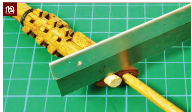
12. Once you are happy with the fit, glue the parts together. When the glue is fully set, cut the excess off the bowsprit and sand the end smooth. Touch up the end of the bowsprit with walnut wood stain.
