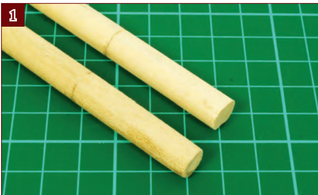
1. Sand two flats on the 10-mm dowel using your original test piece as a guide. (Refer to Stage 41 for instructions on how to fit the dowel if you do not have the test piece.) Make sure that the dowel slides into the socket easily.
