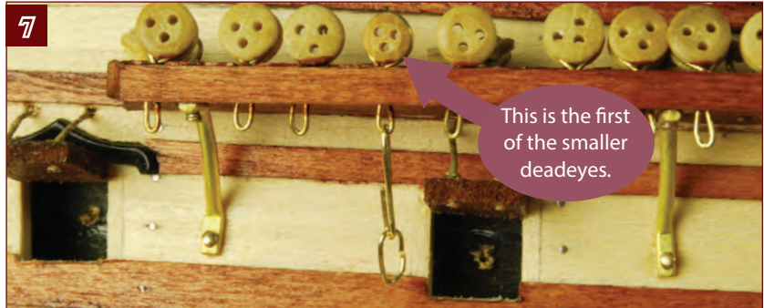
7. Locate the smaller deadeyes on the chainwales. There are 10 on each side of the ship: 4 on the fore chainwale, 2 on the main chainwale, 2 on the small chainwale aft of that, and 2 on the small chainwale aft of the mizzen mast chainwale. Hook the larger loops of the straps from Step 6 onto the brass loop under the first of these.
