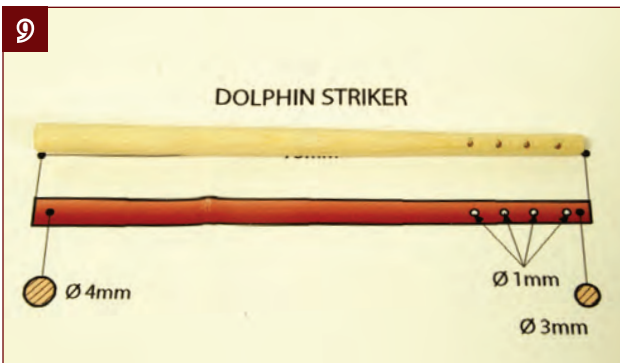
9. Taper the dolphin striker from 4 mm to 3 mm, and drill the four 1-mm holes in the thinner end.
