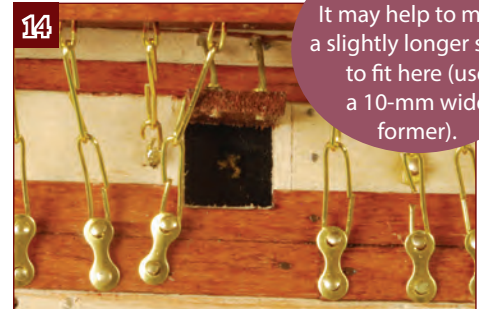
14. Angle the straps forward where you need to clear a gun port.
