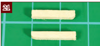
21. Cut two 15-mm lengths of 3 x 3-mm strip. Chamfer one edge so they will fit under the bees, and radius the aft end.
