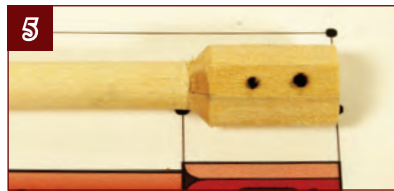
5. Use the 2 x 4-mm wood supplied in this stage to form the octagonal section. The technique is the same as used to construct the yards, so refer to Stage 72 for more details. Then drill the two 1.5-mm holes as indicated.
