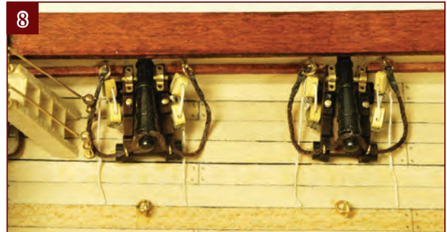
8. Drill 0.7-mm holes in the deck and glue the eyebolts and rings into them about 10 to 12 mm behind each deck gun.
