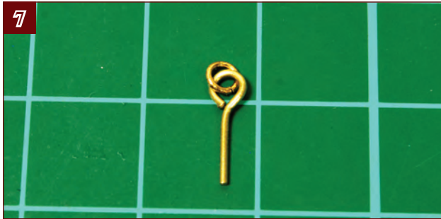
7. Take six eyebolts and six rings. Twist the rings to open them, thread them onto the eyes of the eyebolts, and then close the rings again.
