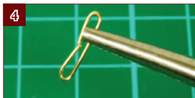
4. Use pliers to flatten the loops into straps. Try the first few in place, as in Steps 7 and 11. You may find you need slightly longer or shorter straps to fit your hull properly, so adjust the wood in Step 2, then make a total of 132 straps.
