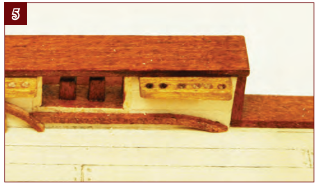
5. Glue the shorter bulwark pin rails near the end of the bulwarks.
