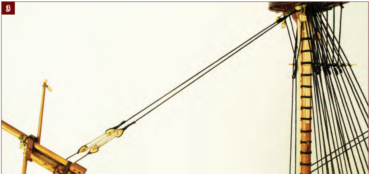
3. The threads should be under a moderate tension, but not so tight that they pull the fore mast or bowsprit out of position.
