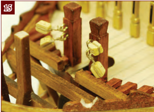
15. Tie the remaining double blocks to the eyes on the knighthead. Leave 1-2 mm of thread between the eye and the block as this will make it easier to thread the blocks.
