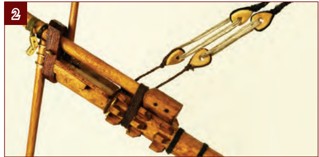
2. The lower ends of the threads are secured to the heart blocks that are already fitted to the bowsprit.
