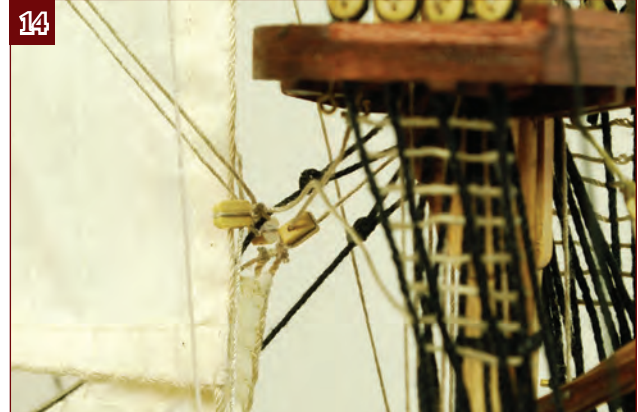
14. Double the threads back on themselves and take them back to the blocks just fitted.
