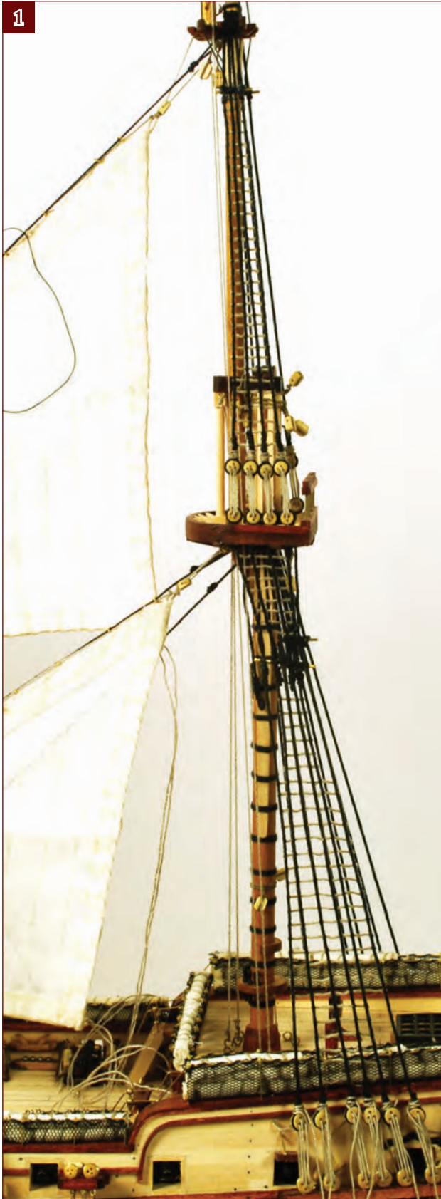
1. The completed mizzen shrouds.
