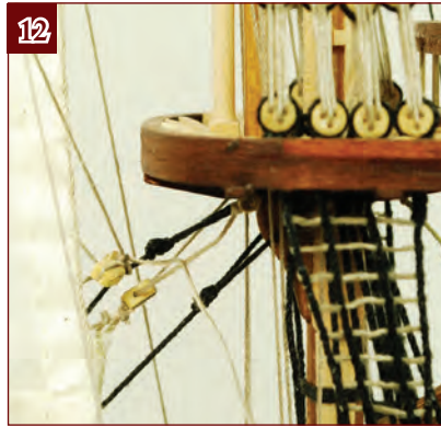
12. Tie the blocks to the stay just below the mizzen top.
