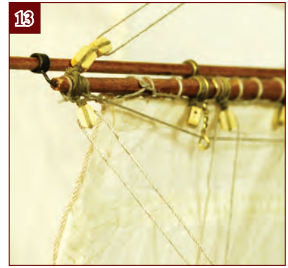
13. Take the long tails up to the blocks on the ends of the yard.
