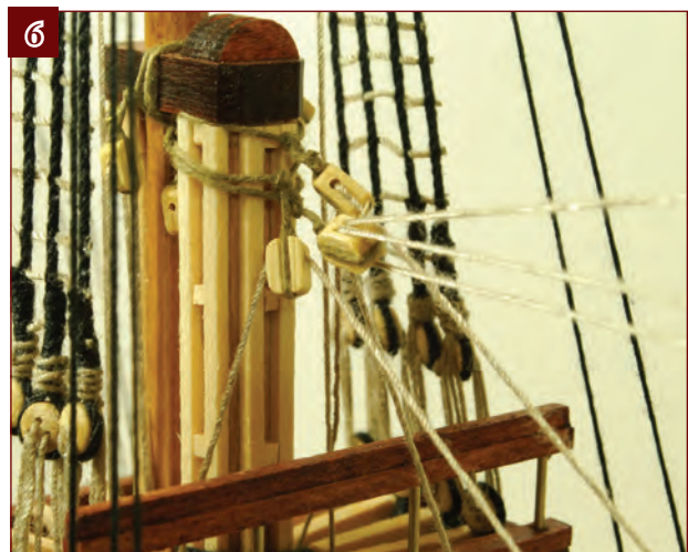
6. Thread it through the single block just below the mizzen mast cap.
