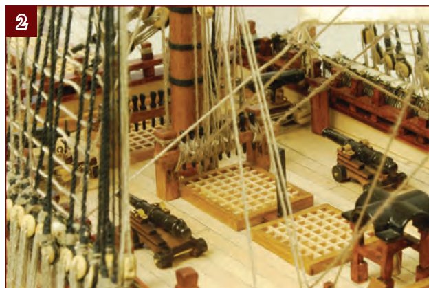
2. Glue the guns to the forward deck using superglue. The rear wheels of the carriages should be in line with the front edge of the rear grating and the guns should be halfway between the grating and the bulwark.
