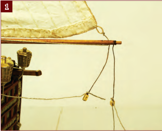
1. Tie 300-mm lengths of thread just above both blocks on the end of the driver boom.
