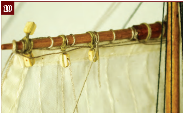
10. Tie a 900-mm length of thread to the yard close to the inner block to form the clew line (C).
