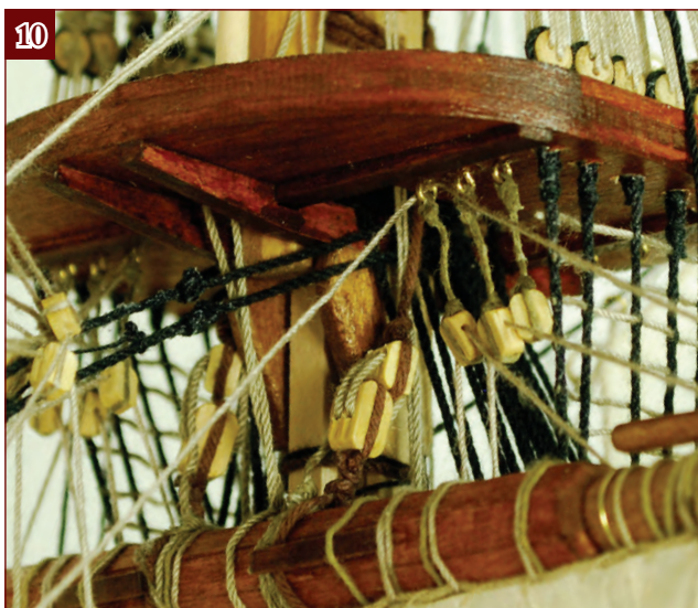
10. Now feed the thread through the inboard eye under the main top.
