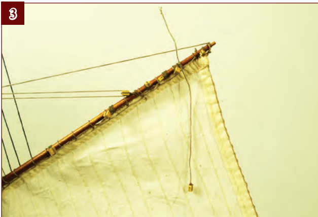
3. Tie a 5-mm single block to some thread, leaving a 150-mm tail. Tie this to the gaff boom next to the double blocks, so that the block hangs down a little over 80 mm from the boom.
