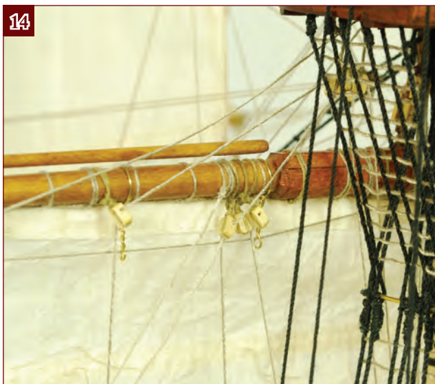
14. Take it back up through the middle of the three blocks.
