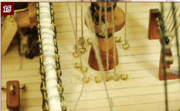
15. Tie the threads off to the front outboard eyes by the mizzen mast. Tension both sides together to make sure the yard stays square.
