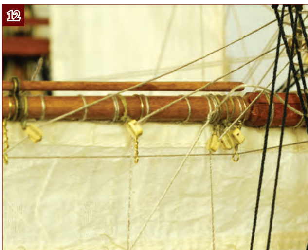
12. Cut an 800-mm length of thread to make the clewline (F). Tie one end to the yard by the group of three blocks.
