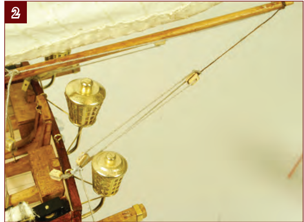
2. Lace each of these threads to one of the single blocks on the outboard eyebolts on the taffrail. Feed the thread through the block on the taffrail, back through the block hanging from the boom, and finally secure the thread to the eyebolt itself.
