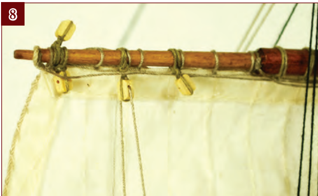
8. Take the buntline under the sail and then back up through the central block.
