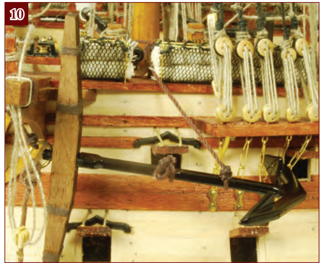
10. Lash the anchor in position as shown, securing the ropes as shown in Steps 11 and 12.
