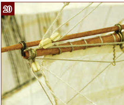
20. Feed this thread through the block on the end of the main yard.
