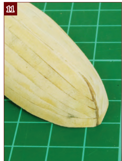
11. Sand the planking at the bow until the stem post shows through. Be careful not to damage the adjacent planks.
