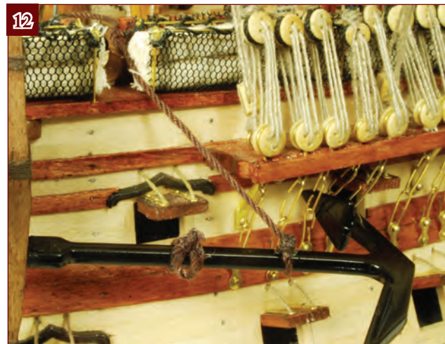
12. Tie the bottom end of the anchor to the timberhead just aft of the carronade. Secure the thread with a clove hitch.
