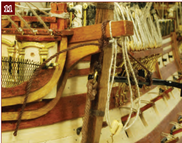
11. Tie the top of the anchor to the cathead. Wrap the thread around the cathead twice and secure it with two half-hitches.
