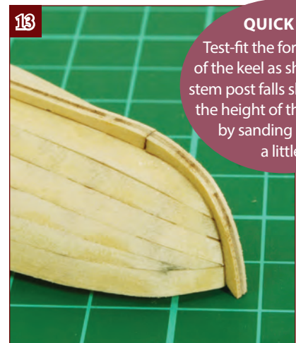
13. Glue the forward part of the keel in place.
