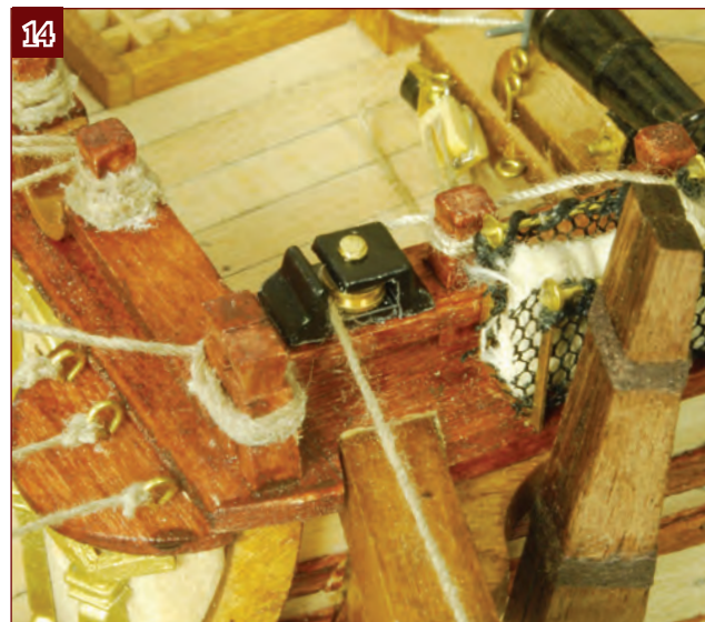
14. Take the thread through the snatch block and secure it to the timberhead aft of the block, using a clove hitch.
