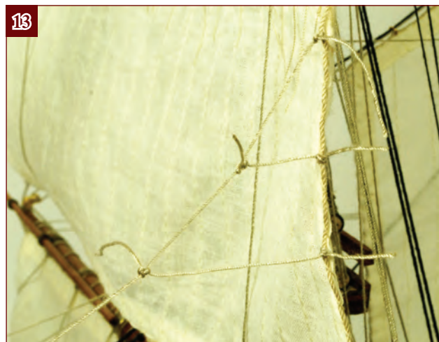
13. Tie an 800-mm length of thread for the bowline.
