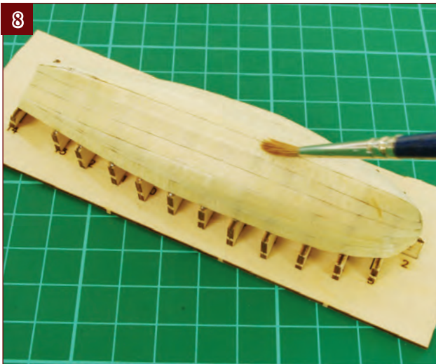
8. Carefully sand the planking smooth and coat it with sanding sealer. Then give it a final light sanding.
