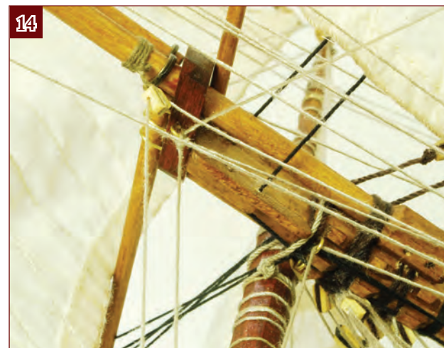
14. Feed this thread through the eyebolt on the bowsprit cap.
