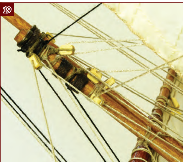
19. Feed the thread through the blocks that were just fitted to the jibboom.
