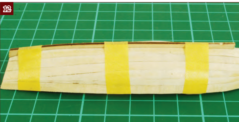
12. Test-fit the main part of the keel, with the rear of the keel aligned with the transom. You may have to sand the bottom of the hull planking to get a good fit. Then hold the main part of the keel in place with tape, and run superglue into the joint. Remove the tape when the glue is dry.
