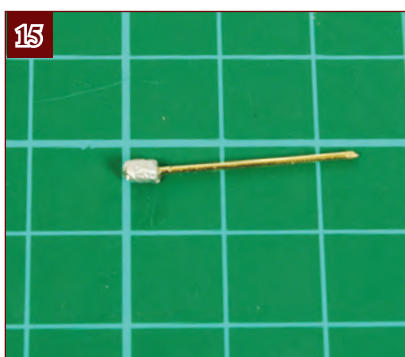
15. Cut a 20-mm length of wire from a large paper clip and glue this into the hole in the sponge swab.
