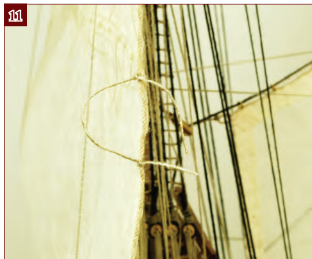
11. To make the fore topsail bowline (C), tie a 20 x 20 mm harness to the sail as before. Align the top of the harness with the bottom reefing band.
