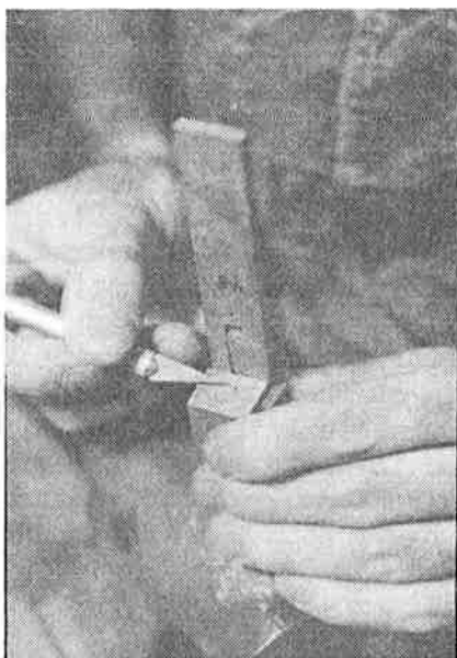
57. Voicing the plectra. This is done from the underside, on a small block of wood.
